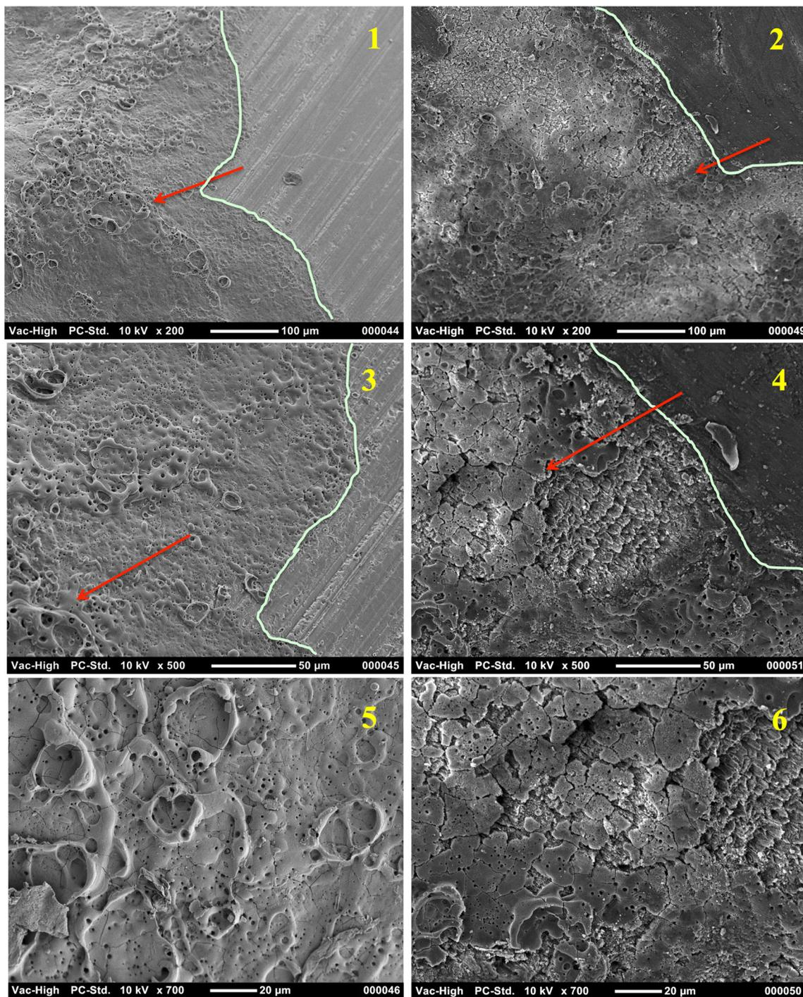
**Fig. 6** Enamel surface after irradiation with 43- $\mu$ s pulse duration. *Left column*, controls with no acid etching; *right column*, after acid etching. SEM of the controls showed homogenous melting with some roughness. Acid etching results in a relatively homogenous pattern with confluent
