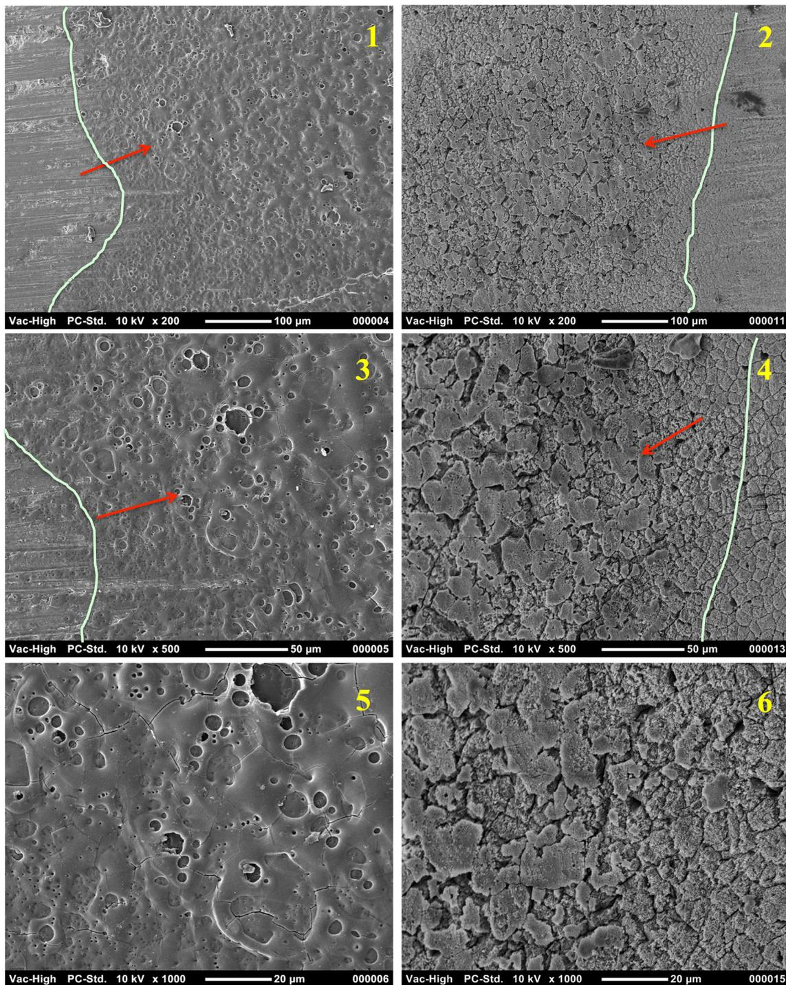
**Fig. 4** Human enamel surface after irradiation with 7- $\mu$ s pulse duration. *Left column*, controls with no acid etching; *right column*, after acid etching. SEM of the controls showed relatively homogenous melting and some minor surface roughness with no surface loss. Acid etching
