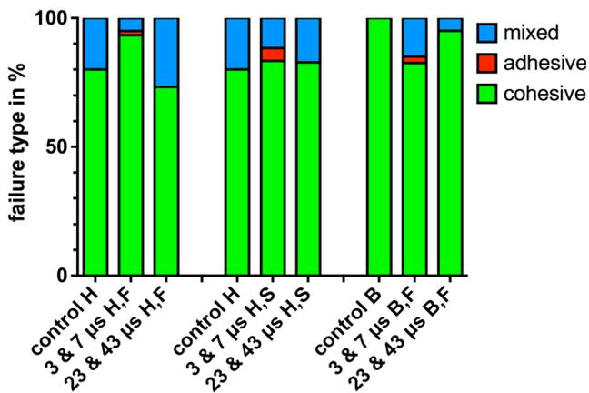
**Fig. 2** Bonding failure mode for human (*H*) and bovine (*B*) enamel for Adper Single Bond Plus and Filtek Supreme—freehand irradiation (*F*) and computerized motor-driven stage (*S*) irradiation. Adhesive, cohesive, and mixed failure in percent. Results separated in control, 3- and 7- $\mu$ s laser irradiation, and 23 and 43  $\mu$ s combined, respectively
