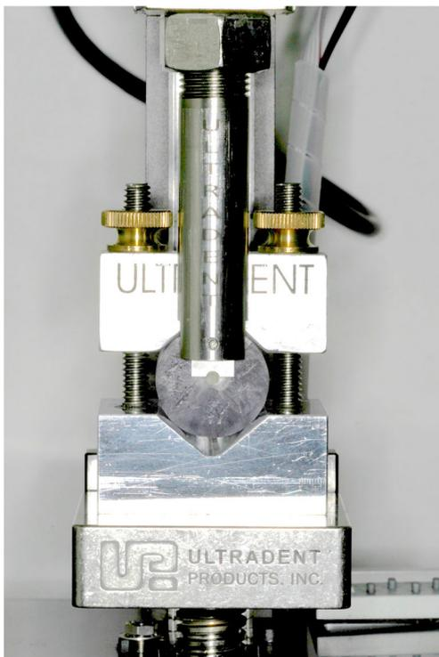
**Fig. 1** Shear bond strength testing machine with the acrylic cylinder secured on a test base clamp, test sample placed under the 2.38-mm notched crosshead assembly
